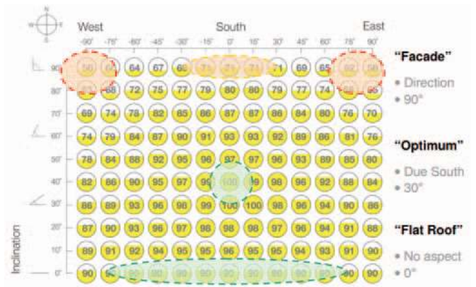
Figure 13: Solar irradiation, azimuth and inclination (image courtesy of solarcentury.com)
